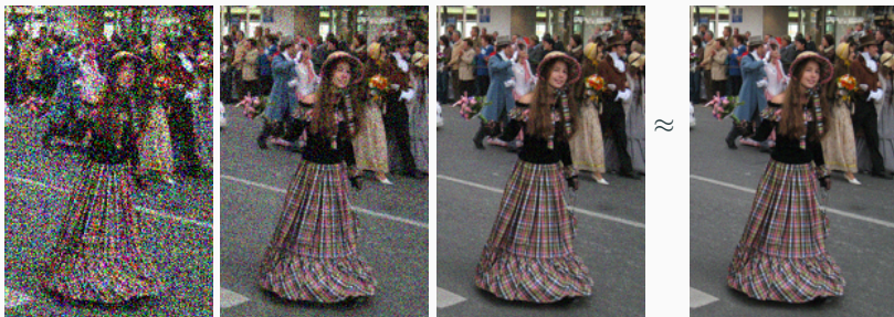
(a) y^k (Gaussian noise) (b) m=9 (SNR \times 3 ) (c) m=81 (SNR \times 9 )
