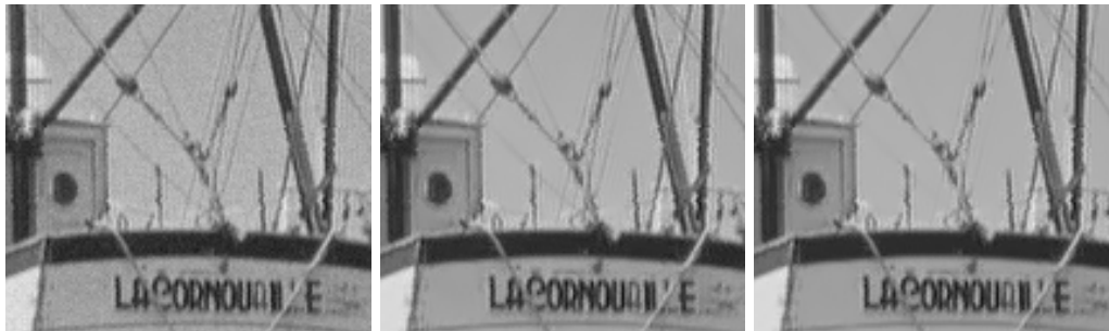
FIG. 2.3. Loss of lines and isolated details. Left: Boat image with little noise ( \sigma = 5 ). Middle: Result of the NLmeans filter ( h = 6 , s^2 = 7 \times 7 , search window 11 \times 11 ). Right: same experiment, using a search window 61 \times 61 . Notice that several ropes vanish when the size of the search window increases (this should be seen on a computer screen).
