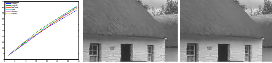
FIG. 4.3. Left: Evolution of the optimal global smoothing parameter h when the noise level \sigma varies, for six different images. The linear behavior is clear. Middle and right: visual difference between the optimal smoothing parameter for this specific image ( h = 14.5 , PSNR = 30,84dB , only an extract is shown) and the optimal one for another image ( h = 16 , PSNR = 30,63dB ): some of the texture was lost.
