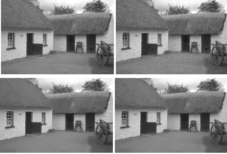
FIG. 4.13. Top left : Original image. Top right: noisy image ( \sigma = 10 ). Bottom left: result of the NLmeans filter ( h = 6.5 , optimized for the PSNR : 30.85dB). Bottom right: result of the local SURE filter (PSNR 31.45dB). The texture of the roof is better preserved, on the ground however the preservation of the texture in small areas looks a bit chaotic.
