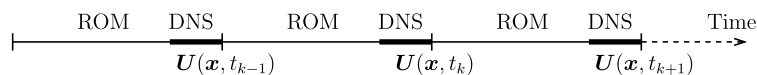
Fig. 24. Schematic representation of the hybrid method DNS–POD ROM to improve the POD subspace.
