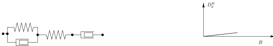
FIG. 24: Burger model: schematic diagramme (left) and plot (right) of plastic flow as a function of tensor B , in the stationary regime and under small applied stresses. In Burger’s model, suitable for foams under low applied stresses (see paragraph III A), the plastic flow increases with the applied stress. If we neglect the short time scale response provided by the Voigt-Kelvin element (spring and viscous element in parallel), then this increase is weak and linear, as determined by the viscous element in series.
