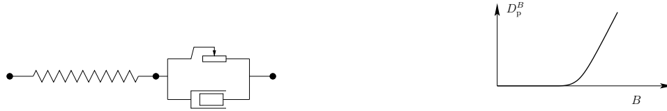
FIG. 25: Bingham model: schematic diagramme (left) and plot (right) of plastic flow as a function of tensor B , in the stationary regime. In a model based on Bingham’s model, such as that developed in the present work, the plastic flow is zero up to a certain stress (yield stress). Beyond the yield stress, it increases (linearly with the applied stress).
