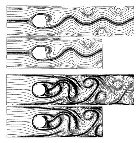
Figure 3. — Stream lines and vorticity lines at Re = 1 000.
