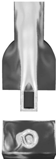
Fig. 6. Adapted meshes: cut through the tetrahedra and associated velocity field (on the top) or curl field (at the bottom).
