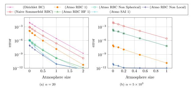
FIGURE 3.  $L^2$  relative errors with reference solution, with respect to the radius of the artificial boundary. The frequency is set to  $f_0 = 30.0$  Hz.
