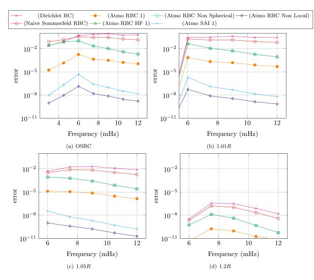
FIGURE 8. L2 relative errors with reference solution, with respect to the frequency. Volumic source with 200 modes.
