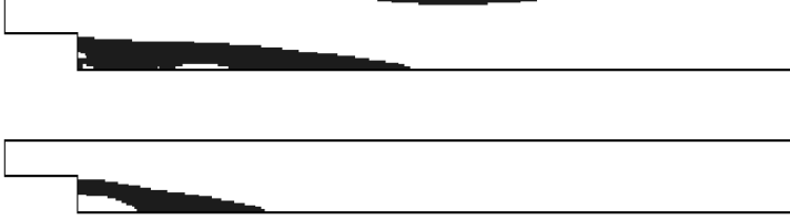
Fig. 15. Mean horizontal velocity u < 0 for uncontrolled (up) and closed-loop (non-intrusive) controlled (down) regime.
