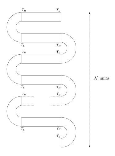
Closed cascade device to generate a pumping effect.
