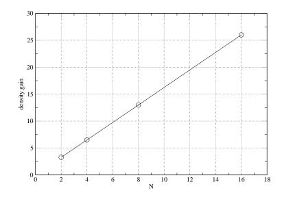
Pressure (left) and density gain (right) for the pumping device with several numbers N of units. Thick case with  $\mathrm{Kn}=0.5$ .
