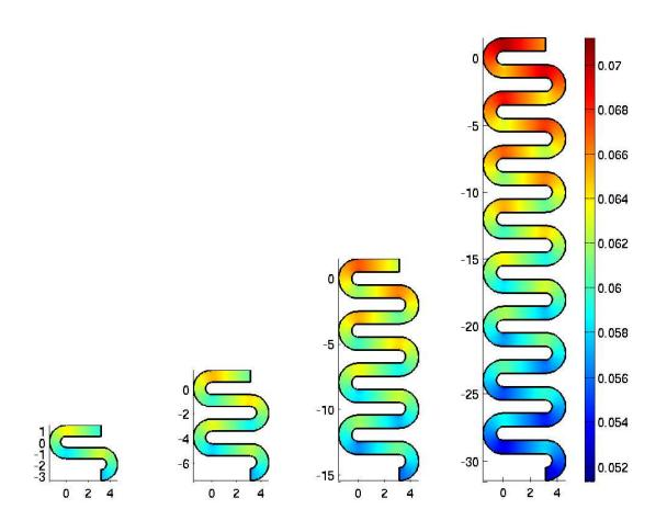
Pressure fi eld in the closed cascade device: 2, 4, 8 and 16 units.
