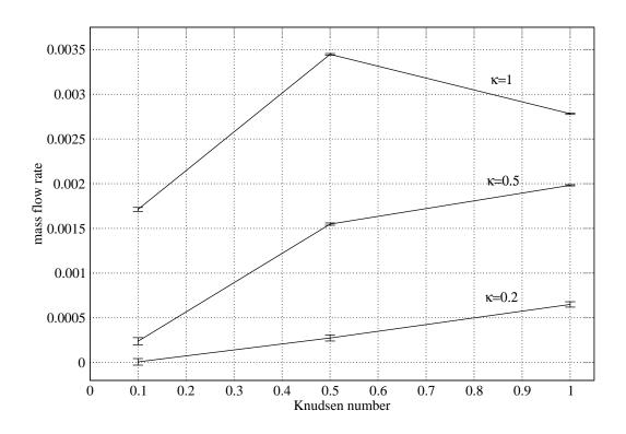
Mass fbw rate in the ring-shaped channel as a function of the Knudsen number.
